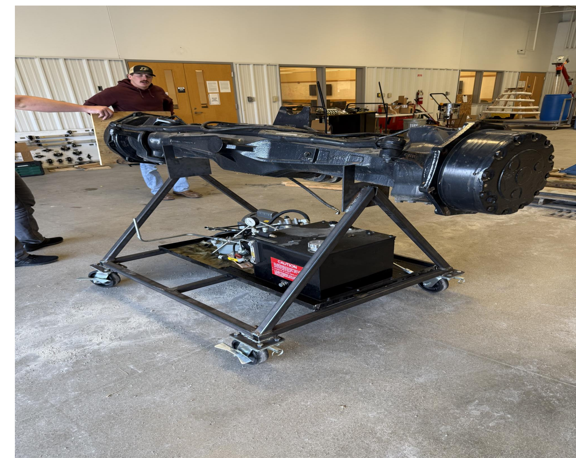
Axle sitting on the stand for the first time under the support of only the stand without other support mechanisms.
